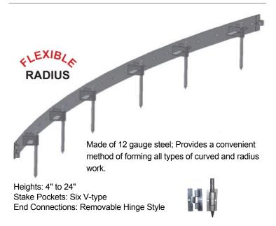
Flexible Radius Concrete Forms are perfect for sidewalks, driveways and other types of paving work. Simply stake the concrete form into the desired position before beginning your pour using the stake pockets and hinge-style stake pocket end connections. The form's durability saves your budget as you reuse your concrete forms again and again. Flexible Radius Concrete Forms are available in heights from 4 inches to 24 inches tall.
