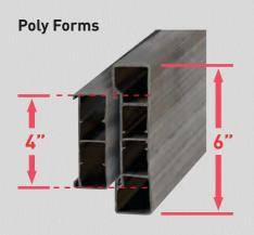
Material: High density Polyethylene (HDPE) Height: 4" and 6" Length: 12' Weight: 4" Flexible - 0.5 lbs. per foot 4" Straight - 1.0 lbs. per foot 6" Flexible - 0.75 lbs. per foot 6" Straight - 1.25 lbs. per foot
